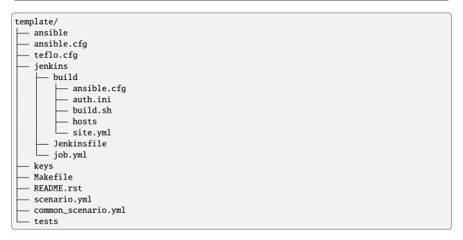
The above scenario structure has additional files that are not required for executing teflo. The extra files are used for easily running the scenario from a Jenkins job. Below are two sections which go into more detail regarding each file.
