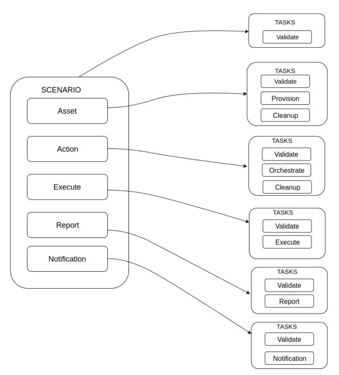
The diagram above shows the teflo object with resources defined. Each of those resources then have a list of tasks associated to it. This means that when teflo runs a scenario, for each task to be processed it will run the given resources associated to that given task.
