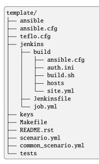
The above scenario structure has additional files that are not required for executing teflo. The extra files are used for easily running the scenario from a Jenkins job. Below are two sections which go into more detail regarding each file.
